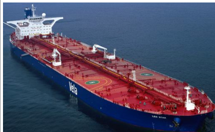
The Leo Star, a double-hulled supertanker capable of transporting 2 million barrels of crude oil, joins the Vela fleet (2002).
